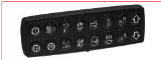
The CL 613/614 keypads have rubber membrane pushbuttons and utilize metal actuation domes for long life exceeding 2 million actuations, HED said. They are offered in two standard form factors — two rows of four buttons or two rows of eight — and are available with a variety of LED colors for each button or indicator. The LEDs are dimmable, both as indicators and icon backlights, HED said, and icons are laser-etched and customizable or available off-the-shelf as circular white icons.
